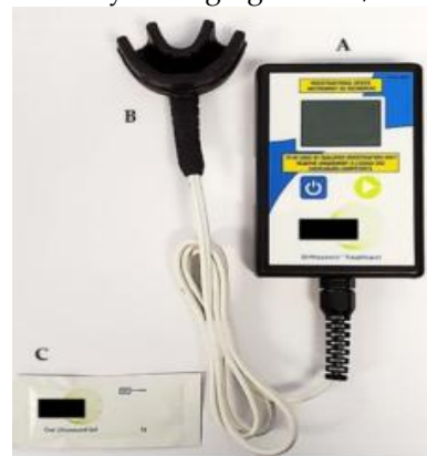
Figure 4. LIPUS device adapted for research. A: Handheld control device. B: Mouthpiece. C: Oral Ultrasound Gel. 14
