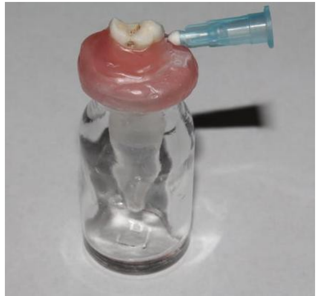
Figure (1). The setup of the experimental device used to test extrusion of debris
